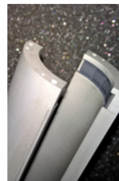
Tomographic ultrasound probe based on cMUT transducers.
